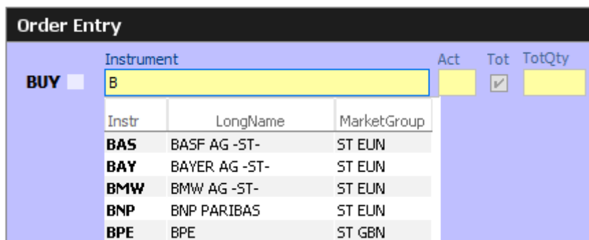
Fig. 12: Text Field Chooser providing a list of values matching the typed string.
