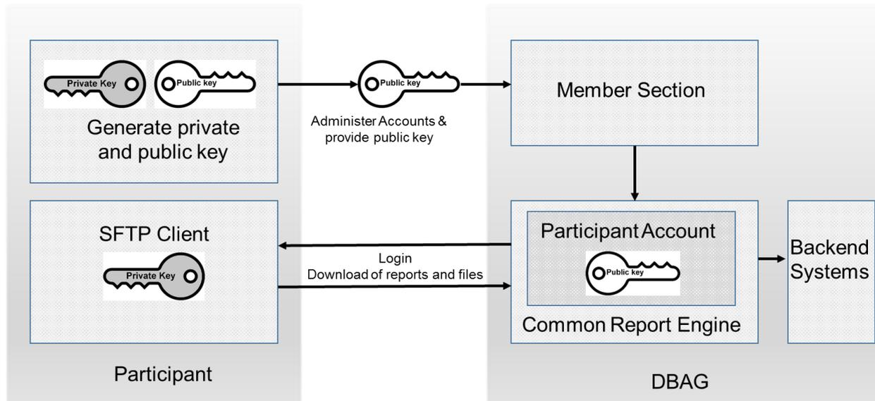
Figure 1: Process overview to connect to the CRE
